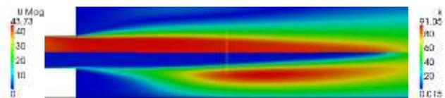
Fig.10. The upper half of figure shows the bulk velocity  $U$  contour and lower half contour is turbulence kinetic energy  $k$
