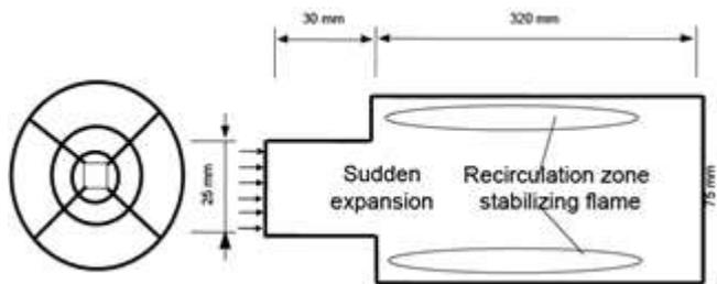
Figure 1b: The problem domain, a co-axial cylinder with turbulence grid in the 25mm-dia cylinder.
