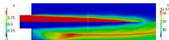
Fig.7. The upper half of figure shows the combustion regress variable  $b$  contour and lower half contour is of turbulence flame wrinkling
