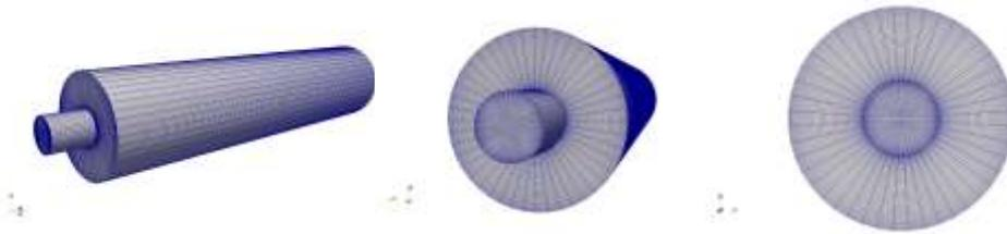
Fig.1a. The mesh of co-axial cylinder (for from L to R: full view, angled view and front view), for dimensions given in Fig. 1b.
