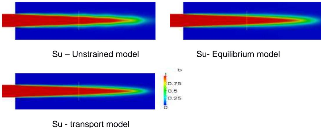
Fig.3 'b' regress variable contours for Xi transport model in combination with three  $S_u$  models, for the equivalence ratio  $\phi=0.5$ . Colour convention blue ( $b=0$ ) is burnt or combustion gas and red ( $b=1$ ) is un-burnt or inlet premixed gas with  $0 < b < 1$ .
