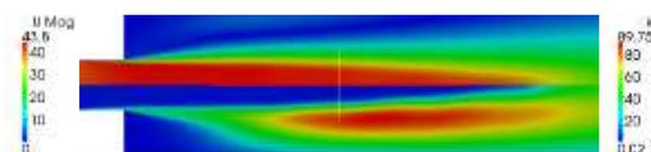
Fig.8. The upper half of figure shows the bulk velocity  $U$  contour and lower half contour is turbulence kinetic energy  $k$
