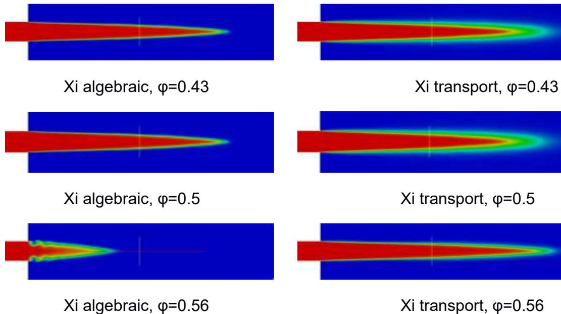
Fig.4 'b' regress variable contours for three equivalence ratios  $\phi=0.43$ ,  $\phi=0.56$  and  $\phi=0.56$  in combination with Xi algebraic and Xi transport models. *Colour convention* blue ( $b=0$ ) is burnt or combustion gas and red ( $b=1$ ) is un-burnt or inlet premixed gas with  $0 < b < 1$ .
