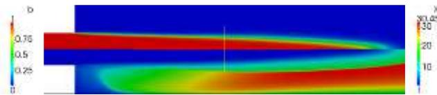
Fig.9. The upper half of figure shows the combustion regress variable  $b$  contour and lower half contour is of turbulence flame wrinkling
