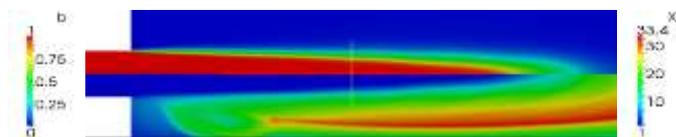
Fig.5. The upper half of figure shows the combustion regress variable  $b$  contour and lower half contour is of turbulence flame wrinkling
