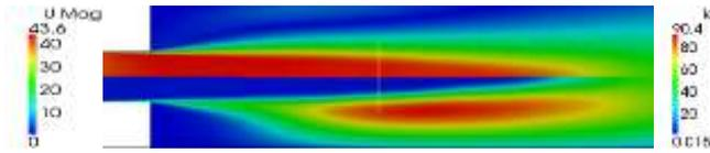
Fig.6. The upper half of figure shows the bulk velocity  $U$  contour and lower half contour is of turbulence kinetic energy  $k$
